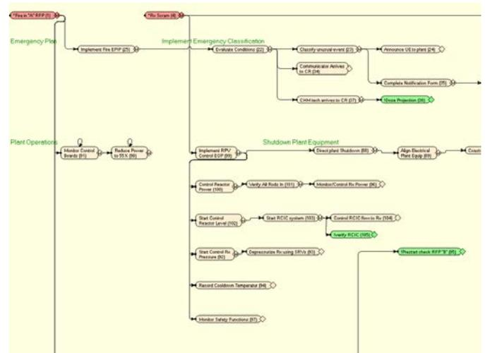
Figure 1 – A portion of the Nuclear Power Plant Human Performance Model
